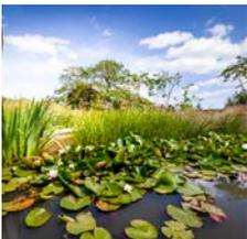
A series of ponds were created which are sustainably designed to take water from the roof of the building and store it. The rainwater filters naturally from the high point of the pond on the Piazza, down the side of the Auditorium to the lower holding pond at the side of the Library and Streatham Farm.
