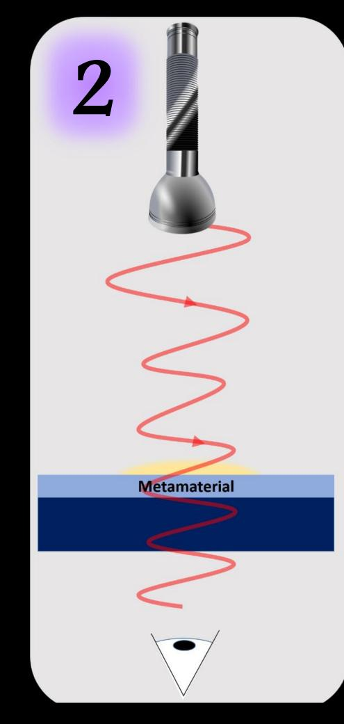
One way to overcome this is to design a 'metamaterial', a special metallic structure, that shrinks the length of the wave.
